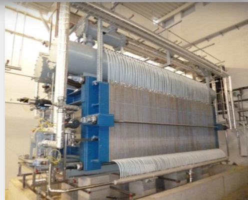
One of three 2 MW Electrolysers
