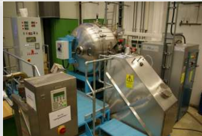
Melt spinning device at IFAM-Dresden
