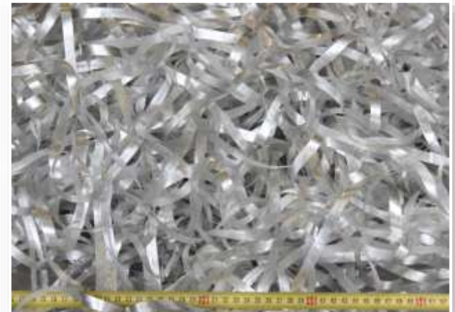
Nanocrystalline ribbons (thickness ~30 \mu\text{m} )
