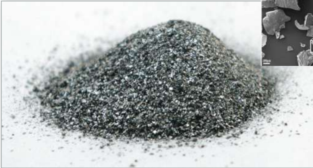
Chopped melt-spun flakes (thickness ~30 \mu\text{m} ; width < 1 mm)
