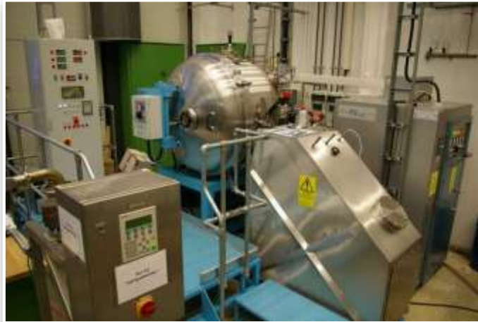
Melt spinning device at IFAM-Dresden
